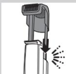
The appliance comes with a comb that allows you to trim hair to different lengths as it keeps the trimming head at a certain distance from your skin. This distance determines the remaining hair length and can be adjusted by turning the zoom wheel. Start at the highest setting to acquire practice with this appliance.
