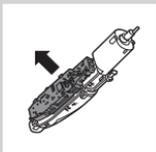
**13** Remove the motor unit from the appliance and remove the battery.
