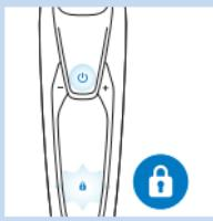
► While you activate the travel lock, the travel lock symbol lights up white continuously. When the travel lock is activated, the shaver produces a sound and the travel lock symbol flashes.
