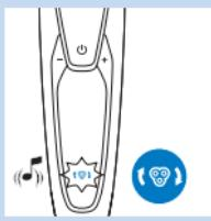
*Note: After replacing the shaving heads, you need to reset the shaver by pressing the on/off button for 7 seconds.*
