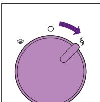
There is a 30 seconds timer for blending function as an overheat protection. If you have not finished blending after 30 seconds, the appliance will switch off and beep twice as a notification. After cooling down for 30 seconds, the appliance beeps once and you can start blending again.
