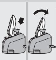
*Note: The shaver cannot be placed in the Jet Clean System when the protection cap is on the shaving unit.*
