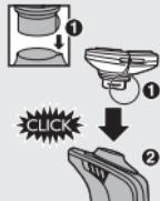
**2 Insert the lug of the new shaving unit into the slot in the top of the shaver (1). Then press the shaving unit downwards (2) to attach it to the shaver ('click').**
