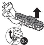
**6** Bend the eight snap hooks aside and remove the cover of the power unit.
