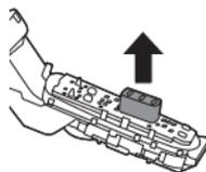
**7** Lift out the two parts of the power unit.
