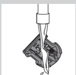
**4 Press the release button (1).The cutting element comes off the appliance (2).**
