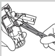
**5** Remove the side panels. Pull the bottom part of the printed circuit board with the rechargeable battery attached from the appliance.
