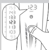
This feature prevents accidental changing of the length setting during trimming. Every time you switch on the appliance, the length setting lock is activated. You can only change the length setting if you switch off the appliance.
