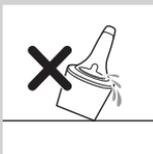
Do not tilt the SmartClean system to prevent leakage.
