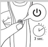
You can lock the shaver when you are going to travel. The travel lock prevents the shaver from being switched on by accident.
