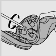
**2** Let the shaver run until it stops and undo the two screws at the back of the shaver.
