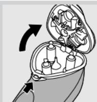
**2** Press the release button to open the shaving unit.
