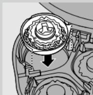
**4** Remove the shaving heads and place new ones in the shaving unit. Put the retaining frame back into the shaving unit and turn the lock clockwise.
