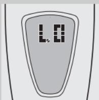
▶ To indicate that the battery voltage is too low to operate the appliance, "LO" appears on the display.
