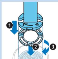
**6** Place the retaining ring holder on the retaining ring (1), place it on the shaving head (2) and turn it clockwise (3) to reattach the retaining ring.
