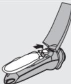
**3** Slide the cartridge with the pump into the shaver. It only fits properly if the white side of the pump is pointing upwards.
