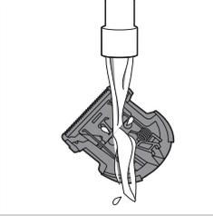
**5** Clean the cutting unit with the brush or rinse it under the tap.
