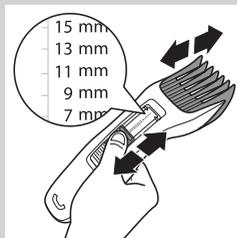
**2** HC3410/17 only: Turn the length setting adjuster to the desired length setting.
