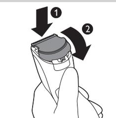
**2** Insert the lug of the new cutting unit into the guiding slot (1) and push the cutting unit back onto the appliance (2).
