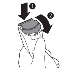
**8** Insert the lug of the cutting unit into the guiding slot (1) and push the cutting unit back onto the appliance (2).
