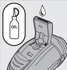
*Tip: For optimal trimming performance, lubricate the trimmer teeth with a drop of sewing machine oil every six months.*
