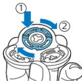
Note: Hold the shaving head holder in your hand when you reinsert the shaving heads and reattach the retaining rings. Do not place the shaving head holder on a surface when you do this, as this may cause damage.
