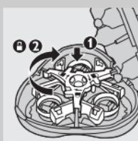
**5** Put the retaining frame back into the shaving unit (1) and turn the lock clockwise (2).
