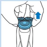
**3** Pull the shaving head holder off the bottom part of the shaving unit.
