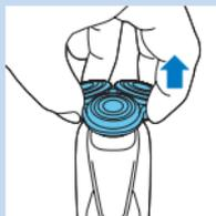
**1** Pull the shaving head holder off the bottom part of the shaving unit.
