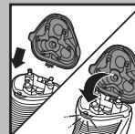
**7** Insert the notch of the shaving unit into the slot in the top of the shaver and then close the shaving unit.
