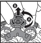
**4** Turn the lock counterclockwise to unlock (A) and remove the retaining frame (B).
