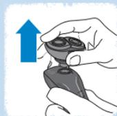
**1** Pull the shaving attachment straight off the appliance. Do not twist.
