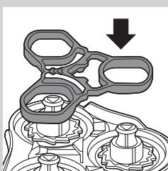
**8** Place the retaining frame back onto the shaving head holder.
