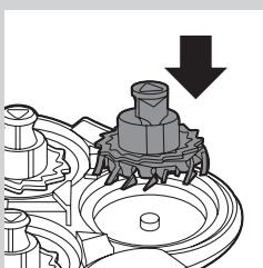
**7** After cleaning, place the cutter back into the shaving guard with the cutter legs pointing downwards.
