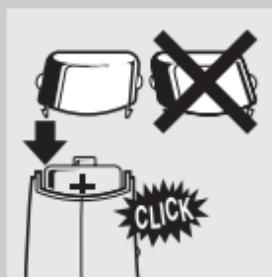
The shaver does not work if the batteries have been placed incorrectly.
