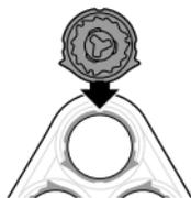
Note: Make sure that the projections of the shaving heads fit exactly into the recesses of the shaving head holder.
