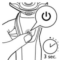
While you activate the travel lock, the travel lock symbol lights up continuously. When the travel lock is activated, the travel lock symbol flashes.
