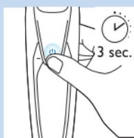
You can lock the shaver when you are going to travel. The travel lock prevents the shaver from being switched on by accident.
