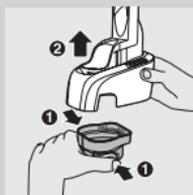
**1** Simultaneously press the release buttons on both sides of the cleaning chamber (1). Then lift the Jet Clean System off the cleaning chamber (2).
