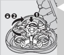
**5** Put the retaining frame back into the shaving unit (1) and turn the lock clockwise (2).
