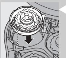
**3** Turn the lock anticlockwise (1) and remove the retaining frame (2).
