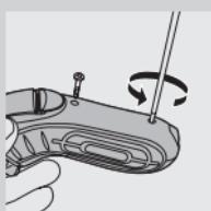
**2** Let the shaver run until it stops, undo the two screws in the hair chamber and remove it.
