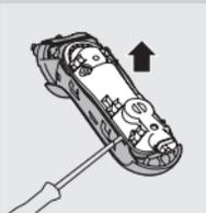
**6** Remove the back panel of the sealed power unit by means of a screwdriver.
