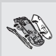
**3** Undo the two screws at the back of the shaver and remove the back panel of the housing.
