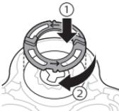
Place the arrows on the ring in line with the projections in the shaving head holder. Turn the ring clockwise until it clicks to indicate that the ring is fixed.
