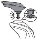
**2** Slide the comb straight into the guiding grooves on both sides of the beard styler ('click').
