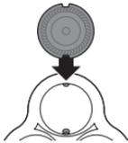
Note: Make sure the notches on both sides of the shaving heads fit exactly onto the projections in the shaving head holder.
