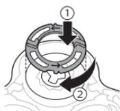
Each retaining ring has two recesses that fit exactly into the projections of the shaving head holder. Turn the ring clockwise until you hear a click to indicate that the ring is fixed.
