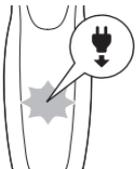
The appliance is equipped with an 'unplug for use' reminder. The 'unplug for use' symbol flashes to remind you that you have to disconnect the appliance from the supply unit before you can switch it on.
