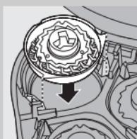
**3** Turn the lock anticlockwise (1) and remove the retaining frame (2).
