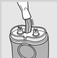
**4** Clean the inside of the shaving unit and the hair chamber with the cleaning brush.
