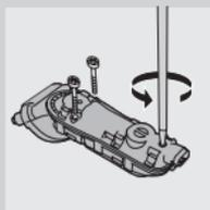
**7** Undo the three screws in the power unit.
