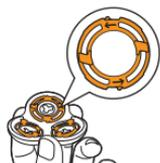
Note: The shaving heads are locked by a blue or an orange retaining ring. Follow the correct instructions.
