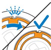
Each retaining ring has two recesses that fit exactly into the projections of the shaving head holder. Turn the ring clockwise until you hear a click to indicate that the ring is fixed.
