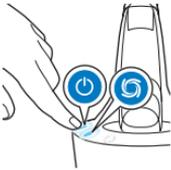
After the rinsing phase, the drying phase starts automatically. During this phase, the drying symbol flashes. When the drying phase is done (after approx. 4 hours), the drying symbol goes out.
