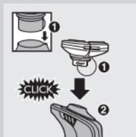
**7** Insert the lug of the shaving unit into the slot in the top of the shaver (1). Then press the shaving unit downwards (2) to attach it to the shaver ('click').
