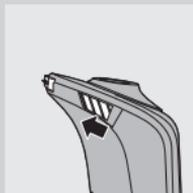
**3** Press the trimmer slide forwards to slide out the trimmer.
