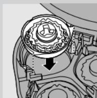
**3 Put the shaving heads back into the shaving unit. Put the retaining frame back into the shaving unit and turn the lock clockwise.**
