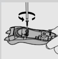
**6** Remove the power unit cover by means of a screwdriver.
