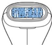
Note: A contaminated light exit window can look like this picture. Make sure you clean the appliance before and after each use and, if necessary, also during the treatment according to the instructions in this section.
