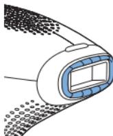
**Note:** The safety ring has contact switches that together are the safety system of the appliance. This safety ring prevents unintentional flashing without skin contact.
