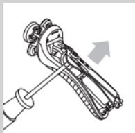
**3** Remove the back panel of the housing with a screwdriver.
