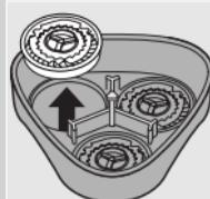
**3** Turn the wheel anticlockwise (1) and remove the retaining frame (2).
