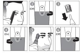
Make sure the guard slides into the grooves on both sides of the trimmer.
