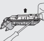
**7** Remove the back panel of the sealed power unit by means of a screwdriver.
