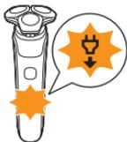
The 'unplug for use' symbol flashes to remind you to disconnect the appliance from the wall socket and remove the small plug from the appliance before you switch it on.
