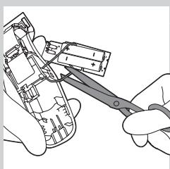
**6** Cut the wires to separate the rechargeable batteries from the appliance.
