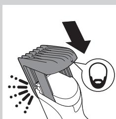
The hair length settings are indicated in millimeters, the comb cuts the hair to a length of 1mm to 23mm. The settings correspond to the remaining hair length after cutting.
