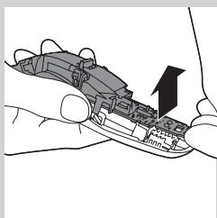
**5** Remove the side panels. Pull the bottom part of the printed circuit board with the rechargeable batteries attached from the appliance.
