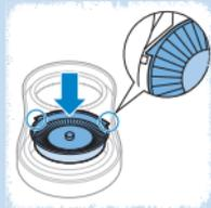
**8** After cleaning, place the shaving guard back into the shaving head holder. Make sure the two wings fit exactly into the recesses of the shaving head holder.
