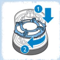
**10** Place the retaining ring back onto the shaving head holder (1). To reattach the retaining ring, turn it against the direction of the arrows indicated in and on the retaining ring (2).
