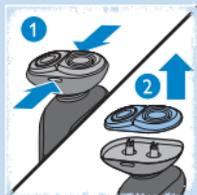
**4** Press the release buttons on the shaving attachment (1) and pull the shaving unit off the shaving attachment (2).
