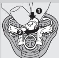
**5** Put the retaining frame back into the shaving unit, press the wheel (1) and turn it clockwise (2).
