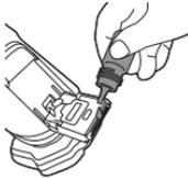
**Tip:** For optimal performance, lubricate the teeth of the pop-up trimmer with a drop of mineral oil every six months (oil not included).
