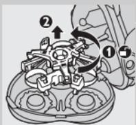
**1** Open the shaving unit, turn the lock anticlockwise (1) and remove the retaining frame (2).
