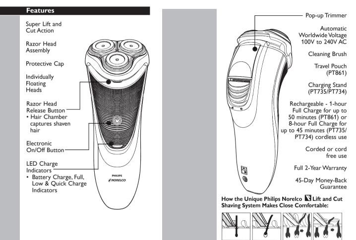
Groove channels beard closer to cutting system Lifter raises hair Slots to cut long hairs
