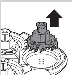
**4** Remove the cutter from the shaving guard.
