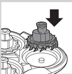
**7** After cleaning, place the cutter back into the shaving guard with the cutter legs pointing downwards.
