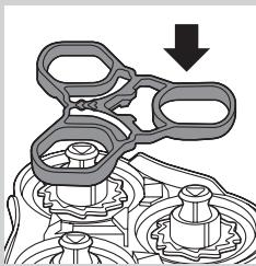
**8** Place the retaining frame back onto the shaving head holder.
