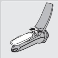
**4** Slide the cartridge with the pump into the shaver. It only fits properly if the white side of the pump is pointing upwards. Close the cover.
