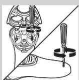
Only remove the rechargeable battery when you discard the shaver. Make sure the rechargeable battery is completely empty when you remove it.
